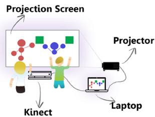
Figure 1: The system structure of POZE.
